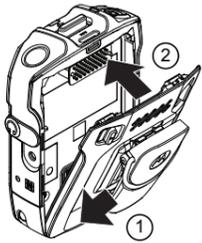
1. Slot in the bottom side of the battery to the RSM battery contact.
