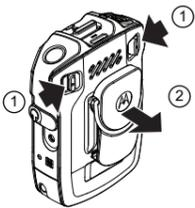
1. Pinch the left and right latches simultaneously.
