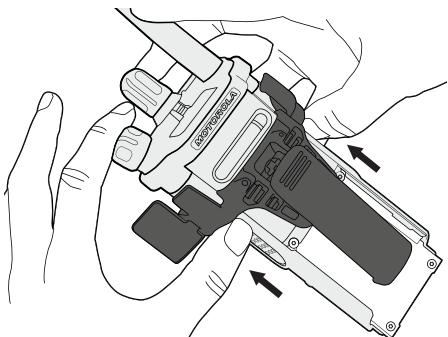
3. Insert the battery. Press on the belt clip for thicker batteries.
