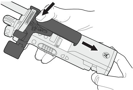
3. Pull the two catches outwards and slide down.
